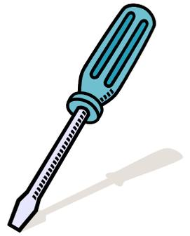
Pay particular attention to the tip size when selecting screwdriver; the tip should fit snugly in the slot of the screw. Do not use a twisted screwdriver tip because it could slip and cause an injury. Never use a screwdriver as a punch, wedge, pinch bar, pry or chisel.
